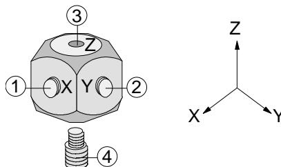
1. Attach the accelerometers for x and y direction by means of the screws ① and ②, which are supplied with the cube. Model 030 has M5 socket cap screws and model 130 has M3 socket cap screws. Model 230 has M8 studs instead. The socket cap screws are freely swivelling inside the cube so that the x and y sensors can be attached in the desired angle position. This can be of advantage with radial cable connectors. Model 230 does not have this feature. \*\*
