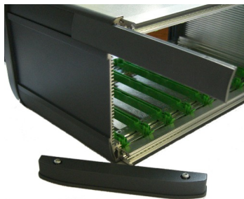
Figure 9: Disassembly of the front cover to attach tower feet
