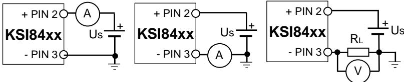
The sensor current can be measured either directly by a current meter connected in series or indirectly by measuring the voltage drop across the load resistance  $R_L$  between PIN 3 and the negative terminal.
