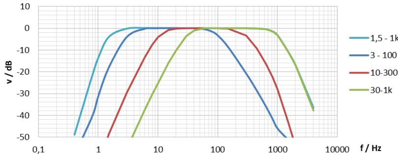
The HP filter of the **displacement** sensor types has a stopband attenuation of -60 dB/decade. The upper cut-off frequency is 300 Hz. It results from the significant decrease of the [dynamic range](#) with increasing frequency. At 300 Hz the maximum current amplitude is only 1 % of the [measuring range](#).
