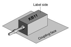
Suitable fixing materials are double adhesive tape, adhesive pads or plastic bonding substances. The softer the adhesive film, the poorer the transmission, especially at high frequencies.
