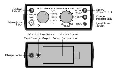
**Power Supply:** Type STV91 works with an internal 9V block battery type IEC 6F22. The battery has to be inserted into the battery compartment at the back of the instrument. It may be operated by a primary battery (that means not chargeable) or a chargeable accumulator (type Ni-Cd or Ni-MH).
