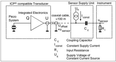
Figure 1: Principle of ICP®
