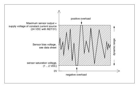
Figure 2: Dynamic range of ICP® compatible sensors
